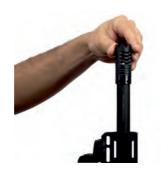
Remove the allens screw with 4-3 number allen key on the handguard
