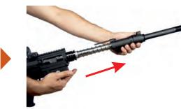
Remove tile takedown pin with a tool to seperate the receivers.
