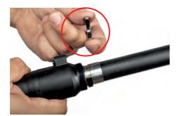
Remove the piston pipe with all other parts which is front side of piston pipe.
